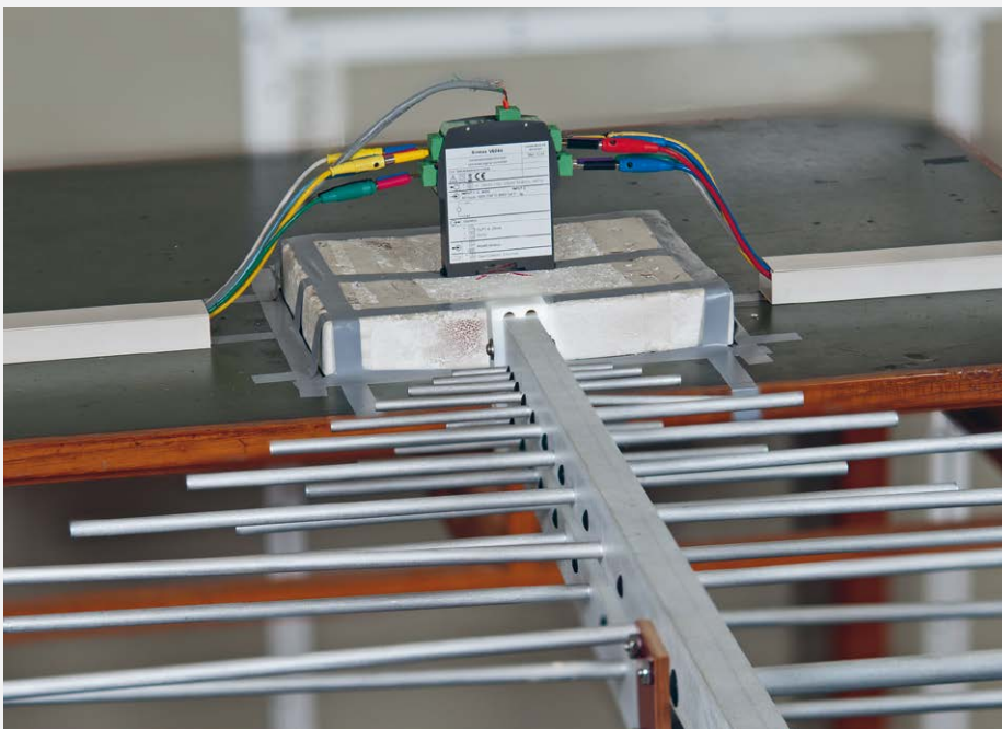
Test of immunity to high-frequency fields on a SINEAX V604s
