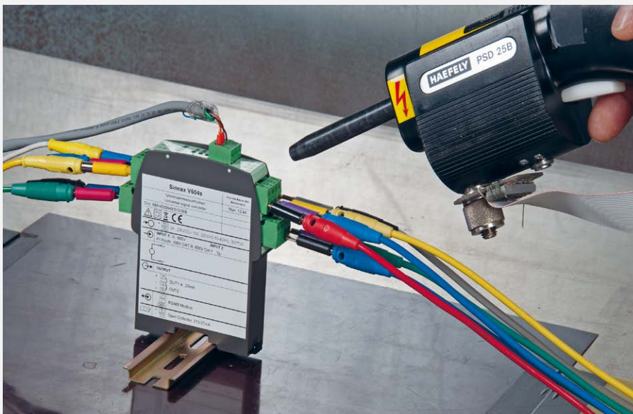
Test of immunity to static discharges on a SINEAX V604s
